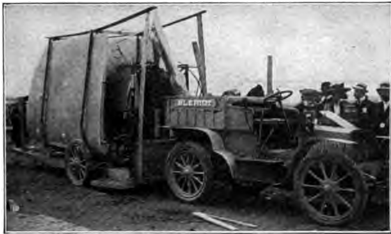
Fig. 50. Portable Bleriot Mounted for Quick Transportation
